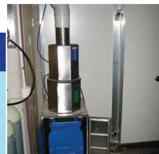
▲ Surf Rock Hotel BottleCycler integrated in bar using chute system to take away empties.
