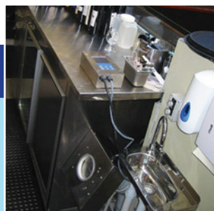
▲ Surf Rock Hotel BottleCycler integrated in bar using chute system to take away empties.
